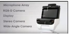
Figure 7: HSR Placement of Cameras and Microphones Source: Toyota Motor Corporation (Toyota 2015)
