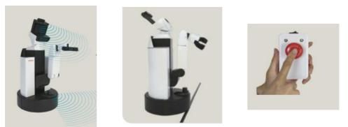
Figure 9: Safety Feature—Obstacle Avoidance Sensors; Magnetic Tape Barriers; Hand-Held STOP Button Source: Toyota Motor Corporation (Toyota 2015)
