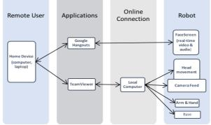
Figure 3: Process for Remote Access of the HSR
