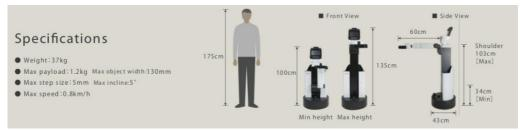
Figure 2: HSR Specifications Source: Toyota Motor Corporation (Toyota 2015)
