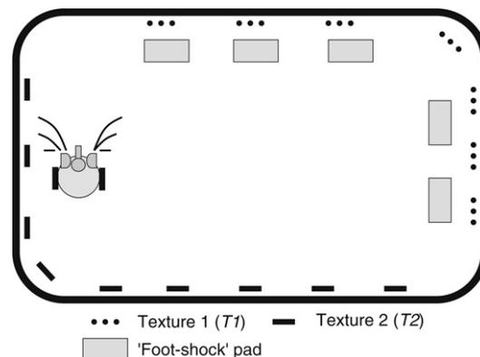
**Fig. 3.** Experimental setup for Darwin IX. Darwin IX explored a walled enclosure (2.41 m × 2.95 m) with textures T1 and T2 on the walls. Instances of each texture were regularly spaced along the walls at intervals of ~30 cm. Located on the floor adjacent to T1 patterns were 'foot-shock' pads made of reflective construction paper. Training and testing was repeated for each Darwin IX subject after exchanging the positions of T1 and T2.
