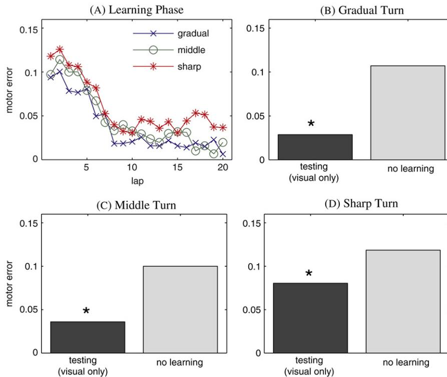
**Fig. 7.** Training and testing the device on different curved courses. The mean motor error from five subjects is shown in the plots. A. Learning curves during training on the gradual turn, sharp turn, and middle turn courses. B–D. Motor errors were significantly lower in the test group, which had access to only visual cues, than in the control or “no learning” groups on the Gradual course (B), Middle course (C), and Sharp course (D). \* denotes  $p < 0.01$  Wilcoxon Rank Sum test.
