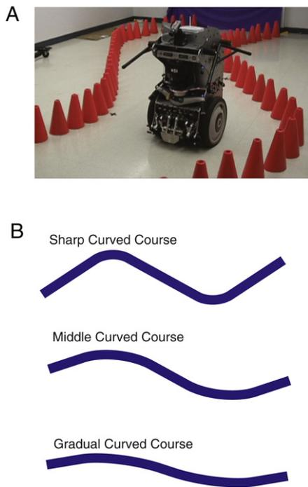
**Fig. 4.** The Segway BBD and its environment. A. The BBD is built on the Segway Robotic Mobility Platform. The device navigated a path dictated by the traffic cones that were spaced apart by a few inches. B. The diagram shows the layout of the different courses. The lane dictated by the cones was five feet wide and roughly 25 feet long. The device itself was approximately two feet in diameter.
