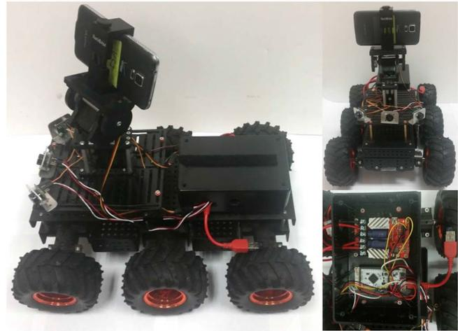
Fig. 5. Android-based robotic platform. Left: side view of ground robot. A flexible pan and tilt unit controls view of smartphone camera. Top right: front view of ground robot. Three LV-MaxSonar sensors are able to detect obstacles up to 254 inches away. Bottom right: top view of component enclosure. An IOIO-OTG microcontroller (below) serves as the central hub for communication, including sending motor commands to the motor controller (above).
