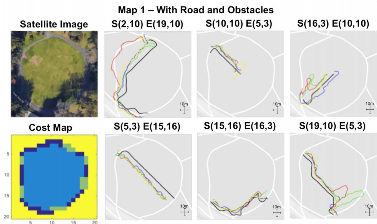
Fig. 9. Experimental results for the spiking path planning algorithm on map 1, with lower costs encoded for the road and higher costs for obstacles. Black lines indicate the planned route and the four colored lines indicate the actual route taken by the robot. Imagery©2016 Google.
