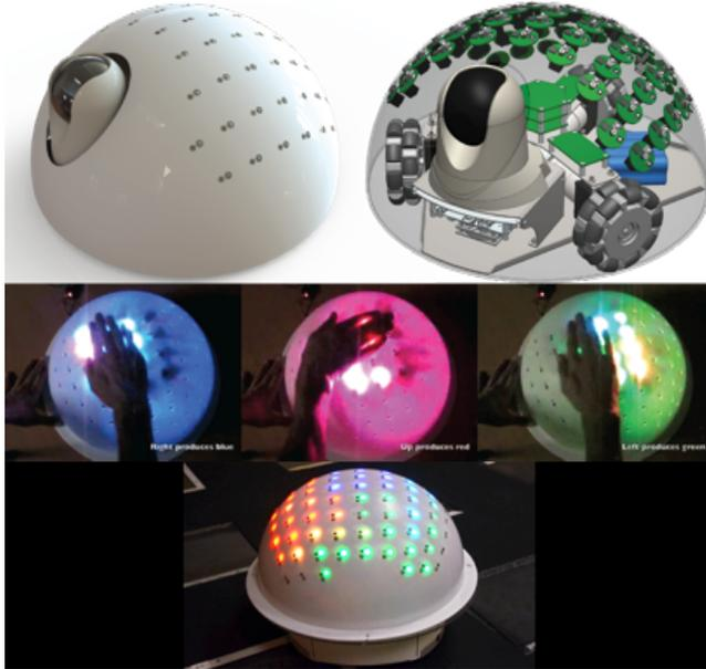
**Figure 1: CARBO. Top left. Rendering shows the trackballs protruding the surface. Top right. Transparent view shows electronics, camera, and drive system. Middle. Example movements and color patterns on the prototype shell. Right movement produces blue, upward produces red, and left produces green. Bottom. The version used in the present study mounted CARBO's shell on an iRobot Create.**
