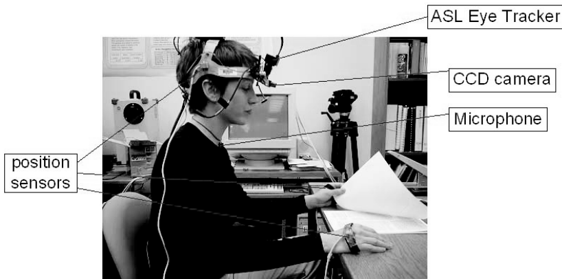
Fig. 4. The computational model shares multisensory information like a human language learner. This allows the association of coincident signals in different modalities.
