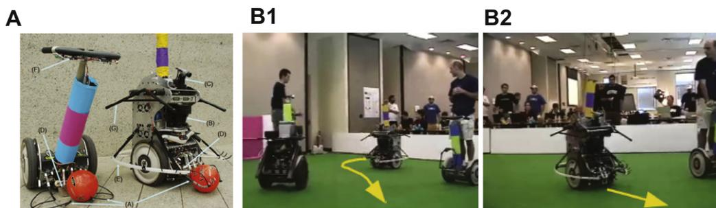
**Fig. 4** (A) The Segway Soccer devices. On the left, a modified Segway HT scooter for the human player. On the right, a brain-based device (BBD) based on the Segway platform. (A) Active capture devices, (B) laser rangefinder, (C) pan-tilt unit and camera, (D) kicking assembly, (E) passive capture ring, (F) voice command module, and (G) crash bars. (B) The Segway Soccer BBD moves downfield through a cluttered playing field toward its opponent's goal. Adapted from Fleischer et al. (2006).
