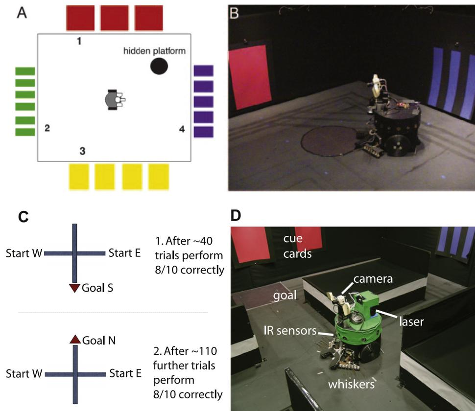
**Fig. 5** (A) Experimental setup for Darwin X, a dry variant of the Morris water maze spatial memory task. (B) Physical instantiation of the spatial memory task. (C) Experimental setup for Darwin XI, a standard plus maze for place learning. (D) Physical instantiation of the plus maze. Adapted from Fleischer et al. (2007) and Krichmar et al. (2005).
