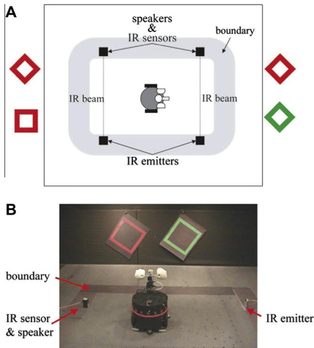
**Fig. 1** Visual binding and categorization in a Brain-Based Device (BBD). (A) Experimental setup. Initially, an auditory cue signaled the brain-based device to orient towards a specific object category. After learning, the BBD oriented towards the object through vision alone. (B) Physical instantiation of the visual binding experiment. Adapted from Seth et al. (2004).
