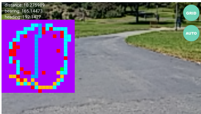
Fig. 6. Screenshot of app used for robot navigation. The screen displays a camera view overlaid with information about distance to the destination, bearing to the destination ranging 0-360 degrees from true north, heading direction (also ranging 0-360 degrees from true north), and the 2D cost grid. Colors on the grid ranging from dark blue to red indicated the costs of the grid, with tree locations marked at highest cost in red. The planned path of the robot is indicated in yellow and the current location of the robot is marked in green. The 'Grid' button toggles the grid view on and off and the 'Auto' button switches the robot into and out of autonomous navigation mode.
