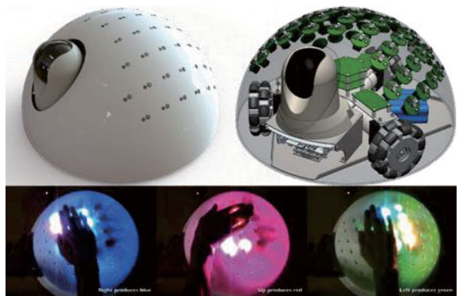
Figure 1. CARL-SJR. Top left. Rendering shows the trackballs protruding the surface. Top right. Transparent view shows electronics, camera, and drive system. Bottom. Example movements and color patterns on the prototype shell. Right movement produces blue, upward produces red, and left produces green.
