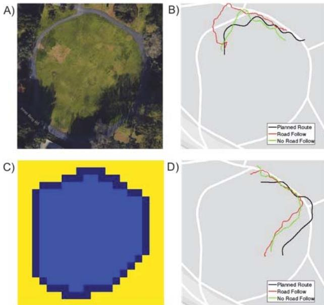
Fig. 3. A) Satellite image of section of Aldrich Park used for mapping. B) Route starting off-road and ending on-road. Black line indicates route assigned by path planner. Red line indicates trajectory taken by road following strategy. Green line is trajectory from original strategy. C) Cost map of area. The road was assigned with a low cost, the middle grass area a medium cost and outer areas high costs. D) Same as B but starting on-road and ending off-road.
