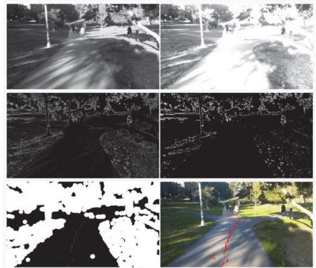
Fig. 2. Road following algorithm. Upper Left: Step 1. Gaussian blur and conversion from RGB to grayscale image. Upper right: Step 2. Contrast and brightness adjustment. Middle left: Step 3. Sobel gradient approximation. Middle right: Step 4. Binary thresholding. Lower left: Step 5. Dilation and path labeling. Lower right: Path display in red on the original test image.
