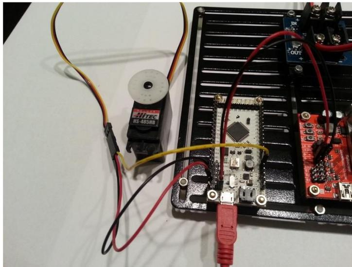
9. Plug battery to Tamiya connector (switch)
