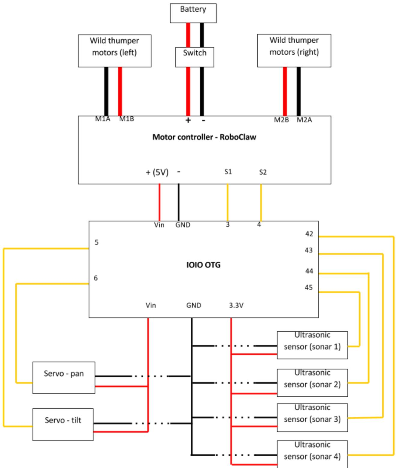
Figure 1. Possible setup of the different components of the ground robot. Schematic not drawn to scale. Thick lines are 14AWG
