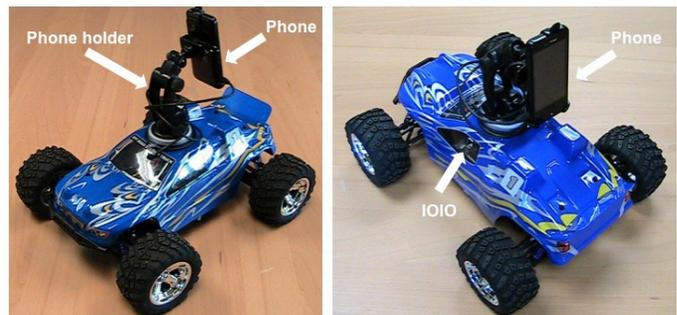
**Figure 1.** The Android Car built using a R/C car, an Android phone, a phone holder and IOIO, could be controlled over Wi-Fi and stream video and sensory information back to a computer. The phone was connected to the IOIO via a USB cable. See Table 2, The Android Car.
