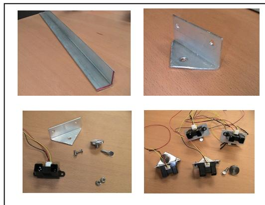
**Figure 4.** Construction phases of mounts for infrared sensors. An aluminum angle was cut and drilled to the dimensions of the IR sensors. Thumbnuts and screws were used to mount the IR sensors to the perforated base.
