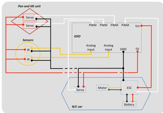
**Figure 5.** Schematic showing the electrical circuitry of the Android based robot. Sensors and actuators are connected to the IOIO except for the motor of the R/C powered by the ESC. Only two sensors are shown here but more can be added to the platform. If more sensors and actuators are used, they should be powered separately (not from the IOIO) since the IOIO can only provide 3A maximum on the 5V output pins.
