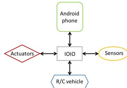
**Figure 2.** Diagram showing the main components of the Android based robotic platform and their interactions. The robotic platform gets sensory input from the phone's internal sensors, as well as external sensors via the IOIO board. The Android phone sends commands to the robot's actuators via the IOIO board. The Android phone interacts with the IOIO board through a USB cable or a Bluetooth connection.
