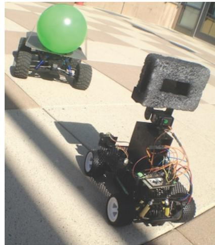
**Figure 8.** Autonomous Android vehicle tracking and following a green ball transported by a remotely controlled vehicle.
