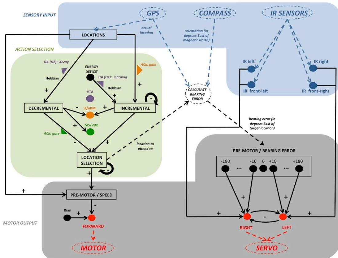
**Figure 9.** Neural architecture driving the behavior of the robot. It was composed of three main groups: sensory input, action selection and motor output. Solid line items represent neural implementation (neurons and connections). See [12] for more details.
