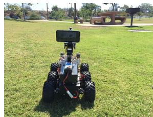
Fig. 1. A six-wheel Android-based ground robot (ABR) used for terrain classification experiments.
