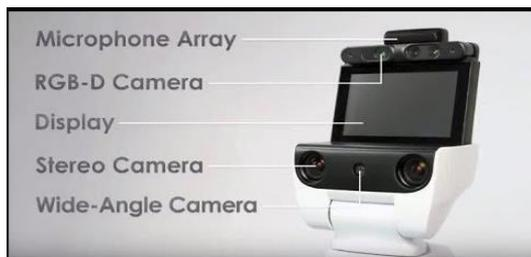
Figure 7: HSR Placement of Cameras and Microphones
