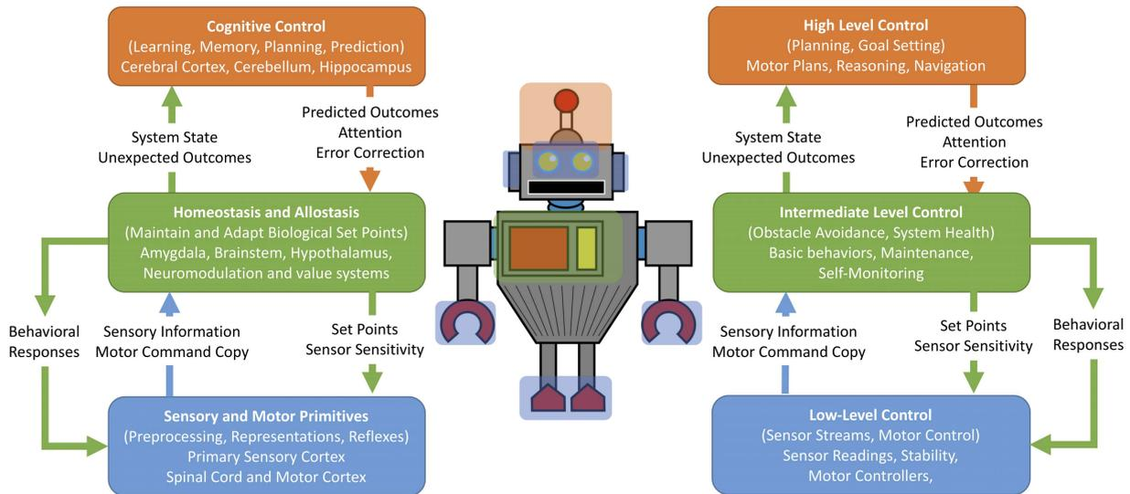
**Fig. 1.** Schematic for neurobiologically inspired autonomous systems. On the left are terms and regions derived from neuroscience. On the right are terms adapted from autonomous robots, but could be applied to many embedded systems. Blue: low-level sensory processing and motor control. Green: homeostasis, maintenance, and monitoring. Orange: high-level planning, adapting, and goal-driven behavior.
