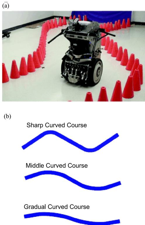
**Fig. 4.** (a) Segway Robotic Mobile Platform navigated a path dictated by orange traffic cones. An adaptive control model based on the cerebellum allowed the robot to learn smooth obstacle-free trajectories through predictive learning. (b) Layout of the different courses. Adapted from [49]. Copyright (2006) National Academy of Sciences.
