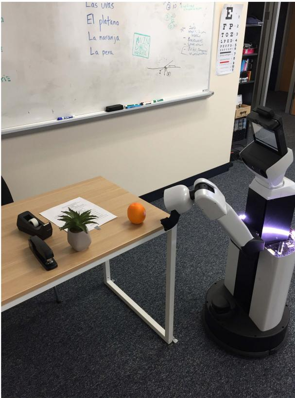
**Fig. 5.** Schema network, from [31] and [68], implemented on the Toyota human support robot (HSR). The HSR retrieved objects in a breakroom and a classroom schema. Search times decreased as the HSR learned which items belong to each schema.
