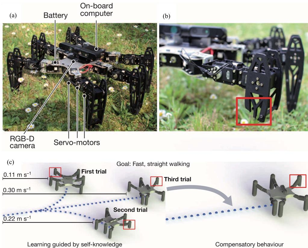
**Fig. 2.** Using an imagined trial-and-error algorithm, robots, like animals, can quickly adapt to recover from damage. (a) Undamaged, hexapod robot. RGB-D stands for red, green, blue, and depth. (b) Hexapod robot with a broken leg. (c) After damage occurs, the robot recognizes that it cannot walk fast and in a straight line. The robot tests different types of behaviors until it discovers an effective compensatory behavior. Adapted from [11]. Reprinted by permission from Springer Nature.
