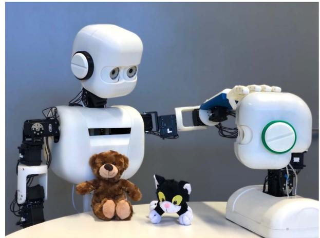
**Fig. 6.** Epi is a humanoid robot developed by LUCS Robotics Group at Lund University in Sweden (<https://www.lucs.lu.se/epi>). It is designed to be used in developmental robotics experiments. The irises of its eyes can change color and the pupils can dilate and contract.
