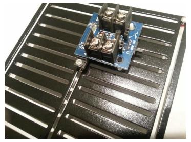
3. mount the motor controller on the plate
