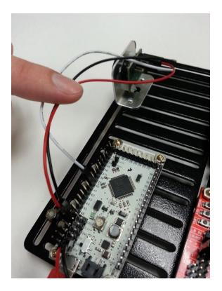
• A HS-485HB servo to the IOIO (5V, GND, PWM pin 5), using male-female wires
