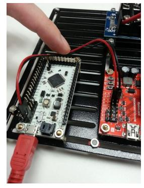
• A sonar to IOIO (3.3V, GND, analog pin 40), using female-female wires
