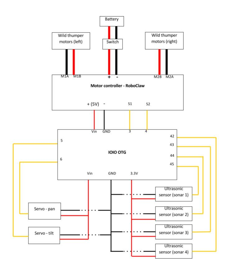
Figure 1. Possible setup of the different components of the ground robot. Schematic not drawn to scale. Thick lines are 14AWG
