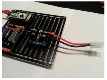
7. Use 14 AWG wires to connect the switch to the motor controller: OUT (+ -) to controller (+ -)
